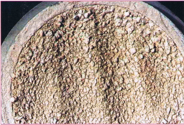
Fig. 8: Filter sample dusted with excellently agglomerating dust from a municipal waste incinerator after cleaning with heavy encrustation
