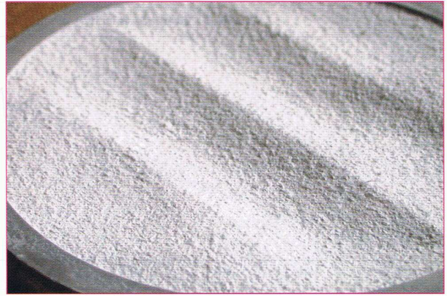
Fig. 9: Filter sample dusted with badly agglomerating dust after cleaning - no pronounced filter cake build-up
