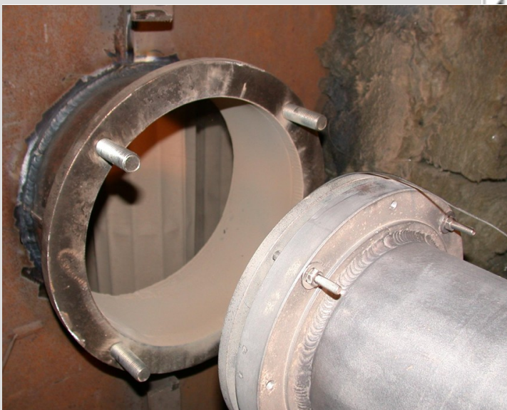
(top) filter probe with heating modules up to 200 °C - (below) filter sample is placed between the filter bags through flange
